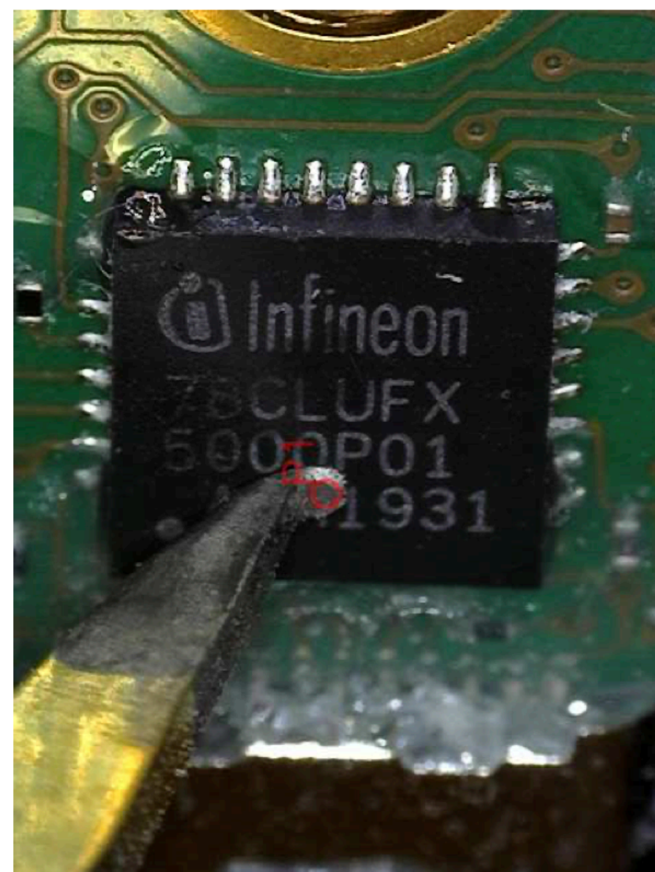
Figure 1.4: YubiKey 5Ci – EM Acquisition Setup
